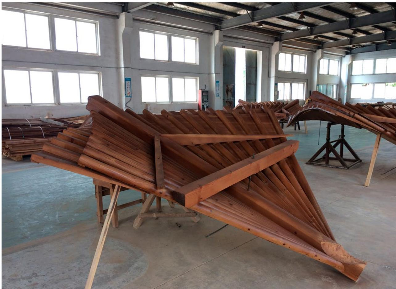
Figure 1-7: Assembled corner roof eaves (supported upside-down) at the Suzhou Garden Development Co. Ltd. Photo by author, 2017.
