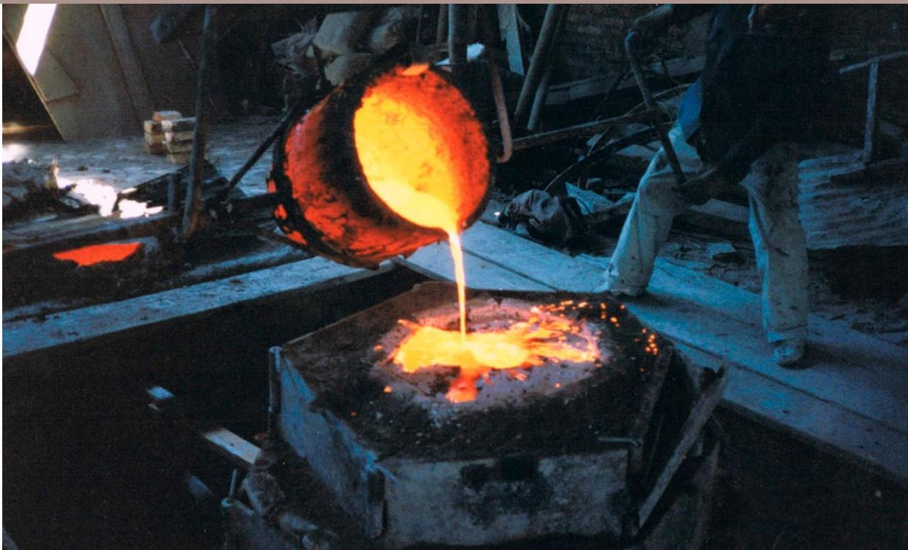
Figure 3-9: The casting process. Photo courtesy of Fred Parhad.
