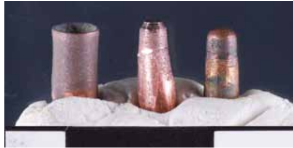
Fig. 14. Experimental tubular and solid copper drills with abrasive.
