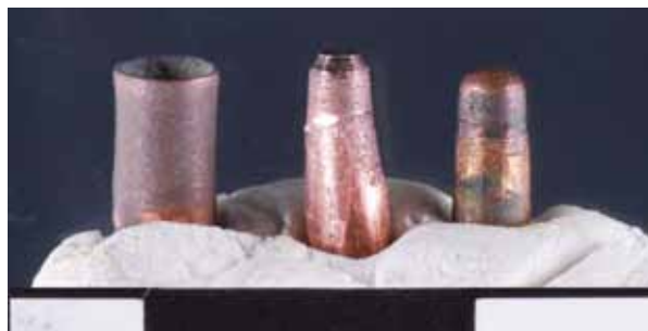
Fig. 14. Experimental tubular and solid copper drills with abrasive.
